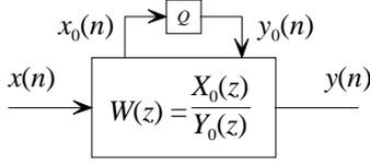
**Fig. 1.** A general nonlinear feedback system with a single quantizer.
