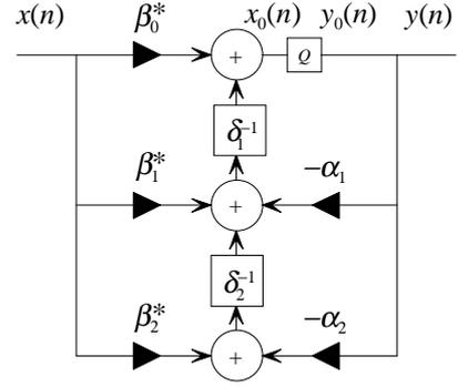
**Fig. 3.** The delta DFII structure. Asterisk (\*) in the coefficients means that scaling is embedded.
