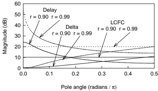
**Fig. 5.** Noise gains of second order DFII structures when  $L_\infty$ -scaling is used. Only one quantization assumed also in delay structure.
