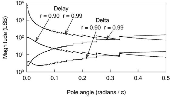
**Fig. 4.** Upper bounds for limit cycle amplitudes of second order DFII sections as a function of the pole angle (note the scale),  $r$  is the pole radius.
