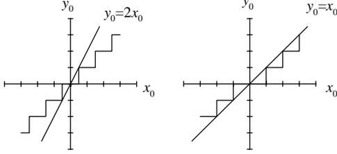
**Fig. 2.** A sector condition for rounding and magnitude truncation quantizers.
