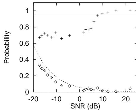
Figure 3: Comparison between theory and experiment for the single-record QPC detector.  $P[\text{hit|QPC}]$ ; theory (solid line) and experiment (crosses).  $P[\text{hit|no QPC}]$ ; theory (dashed line) and experiment (diamonds).
