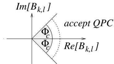
Figure 2: Schematic diagram showing complex bispectrum plane.  $\Phi_c$  defines the critical region inside which  $H_0$  is accepted.
