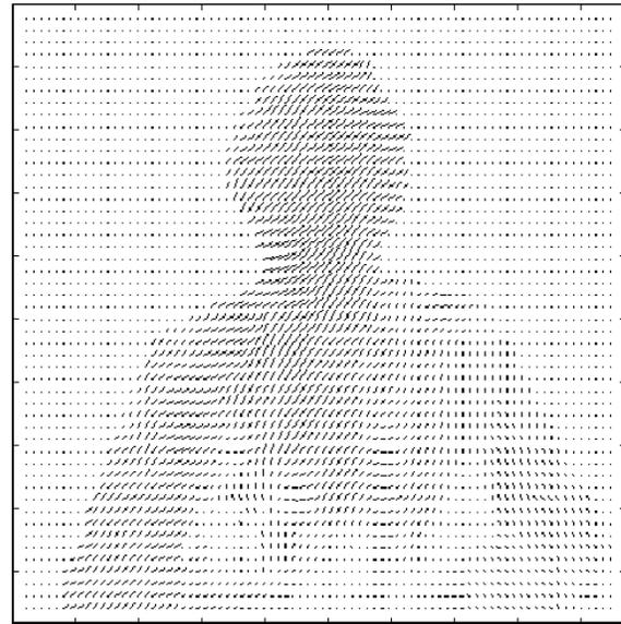
Figure 1: Simulation result with “Trevor White” test sequence: Only one frame and the corresponding displacement field are shown. Only every 4th motion vector is displayed.
