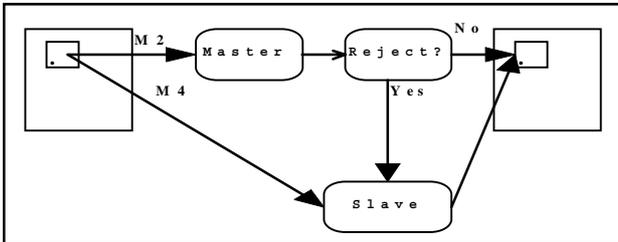
Example of "Master-Slave" architecture with M2 and M4
