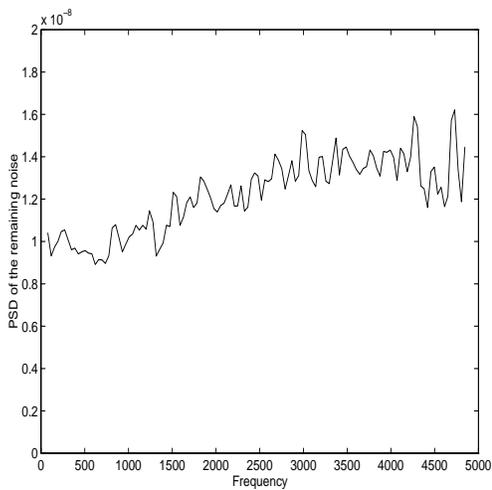
Figure 3: *Estimation of the PSD of the noise resulting from the interpolation of a randomly sampled band-limited noise using a sample-and-hold.*
