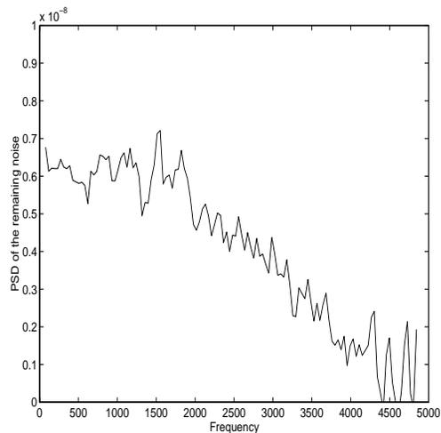
Figure 4: *Estimation of the PSD of the noise resulting from the interpolation of a randomly sampled band-limited noise using a polygonal hold.*
