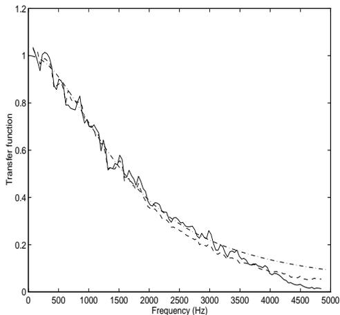
Figure 2: *Transfer function resulting from the interpolation of a randomly sampled band-limited noise. (- -): zero-order, (-.-): modelling, (-): first-order.*
