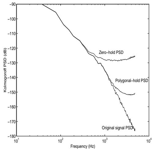
Figure 6: *Estimation of the PSD of a Kolmogorov process.*
