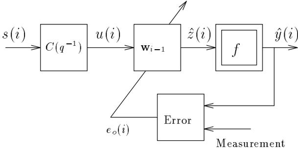
Figure 2: Structure of the nonlinear adaptive equalizer.
