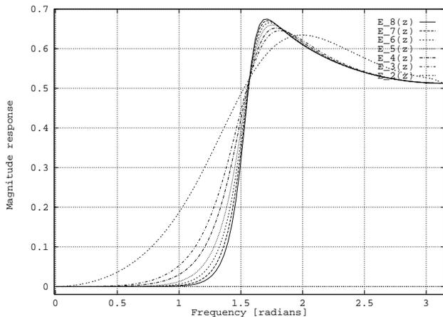
Figure 2: Output error at the low frequency channel.
