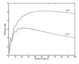
Figure 2: SNR gains on signal containing two damped exponentials at 0 dB. (—) True gain using exact expression of  $f_L(z)$ . (···) Polynomial approximation, m = 30.
