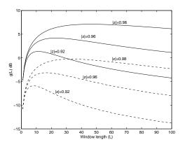
Figure 1: SNR gain versus window length for SNR = 0 dB (—) and SNR = -10 dB (···).
