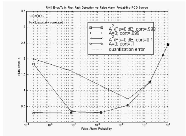
**Figure 6: First arrival RMS detection error as a function of  $P_{FA}$  and for different temporal correlation values and direct path powers.**
