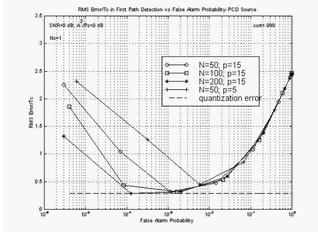
**Figure 5: First arrival RMS detection error as a function of  $P_{FA}$  and data record length. Different values of the assumed duration of the temporal correlation are used.**
