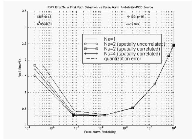
**Figure 4: First arrival RMS detection error as a function of  $P_{FA}$  and the number of sensors, for spatially correlated and uncorrelated sources.**
