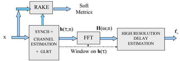
Figure 1: First arrival path detection block diagram.
