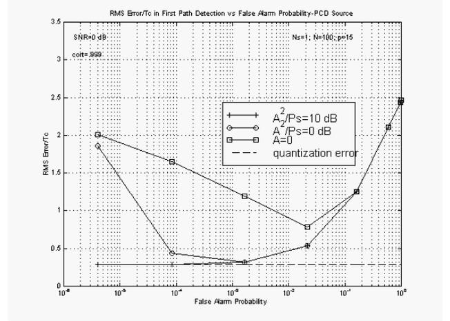
**Figure 3: First arrival RMS detection error as a function of  $P_{FA}$  and for different powers of the direct path. One sensor, and high temporal correlation.**
