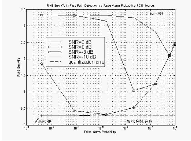
**Figure 2: First arrival RMS detection error as a function of  $P_{FA}$  and for different SNR. One sensor, and a high temporal correlation.**
