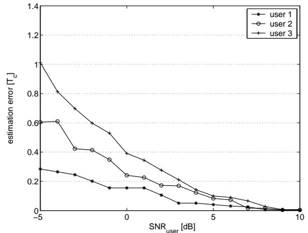
Figure 3: The error in delay estimation vs the SNR
