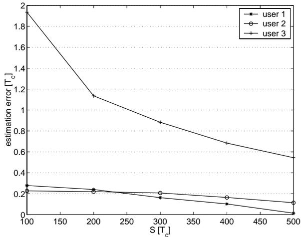
Figure 4: The error in delay estimation vs lag parameter ( $SNR_{user}=5\text{dB}$ )
