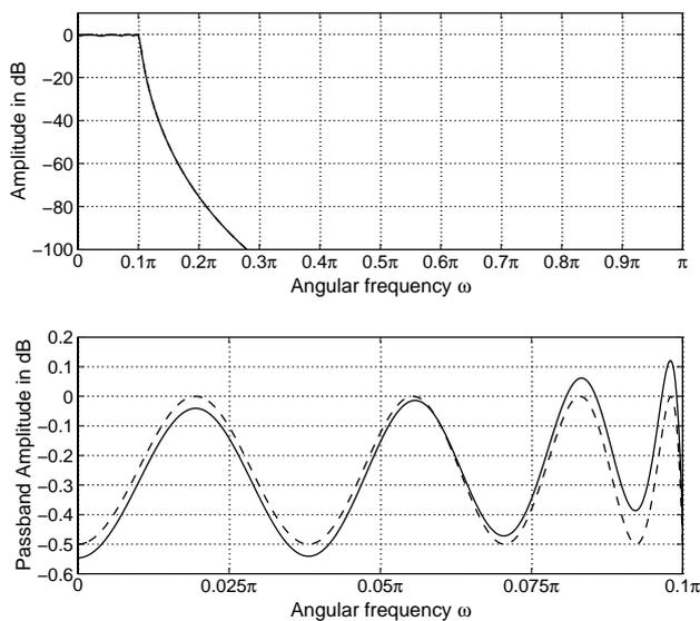
Fig. 2. Amplitude responses in the case of Filter 1 in Table 1 for the infinite-precision filter (dashed line) and for the filter with twenty-four nonzero bits (solid line).
