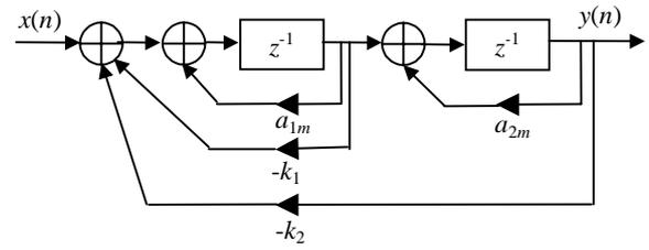
Fig. 1. Modified second-order all-pole section.
