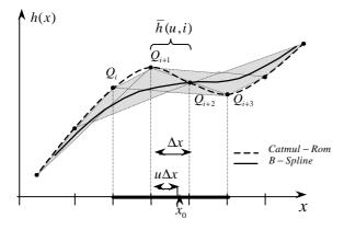
Fig. 4 Cubic-Spline interpolation of control points.
