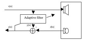
Fig 1. Architecture of a typical echo canceller
