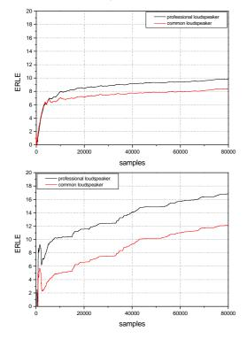
Fig. 3 Measured ERLE for a white gaussian noise and a male voice
