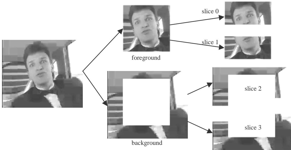
**Figure 1. Example of picture, sub-picture, and slice structures.**
