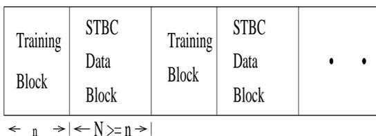
Figure 1: Transmission scheme for fast fading.
