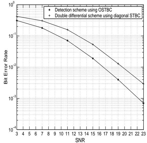
Figure 2: Bit Error Rates for the proposed detection scheme and the scheme in [7]
