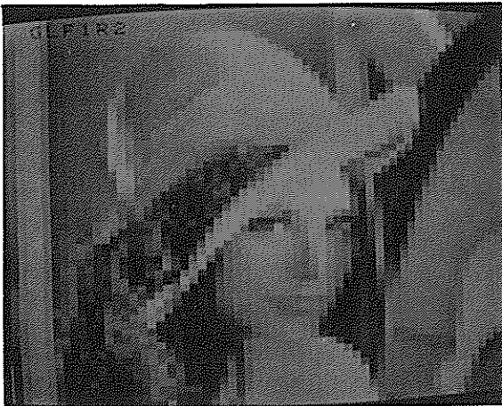
Fig. 2. Reconstructed image of 'Girl', using DFT. Stage II (i.e., [D_8]_{II} ). Bit rate: 1/2 BPP
