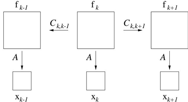
Figure 1: Relationship between high and low resolution frames.
