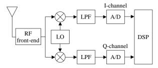
Figure 1: Generalized structure of an I/Q processing receiver.
