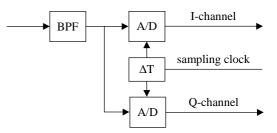
Figure 4: Approximative quadrature sampling to generate the Iand Q-channel signals.
