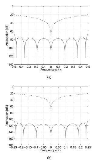
Figure 7: Equivalent image attenuation with (solid) and without (dashed) imbalance compensation for oversampling factors of (a) 2 and (b) 4.
