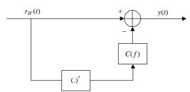
Figure 3: Imbalance compensation structure.
