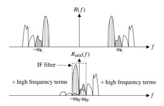
Figure 2: A frequency domain illustration of finite image rejection due to I/Q imbalances. This clearly shows how the imbalances result in a mixture of the desired signal (grey) and the image signal (cross-hatched).
