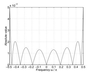
Figure 6: Error in the least-squares optimized compensation filter for oversampling factor of 2.
