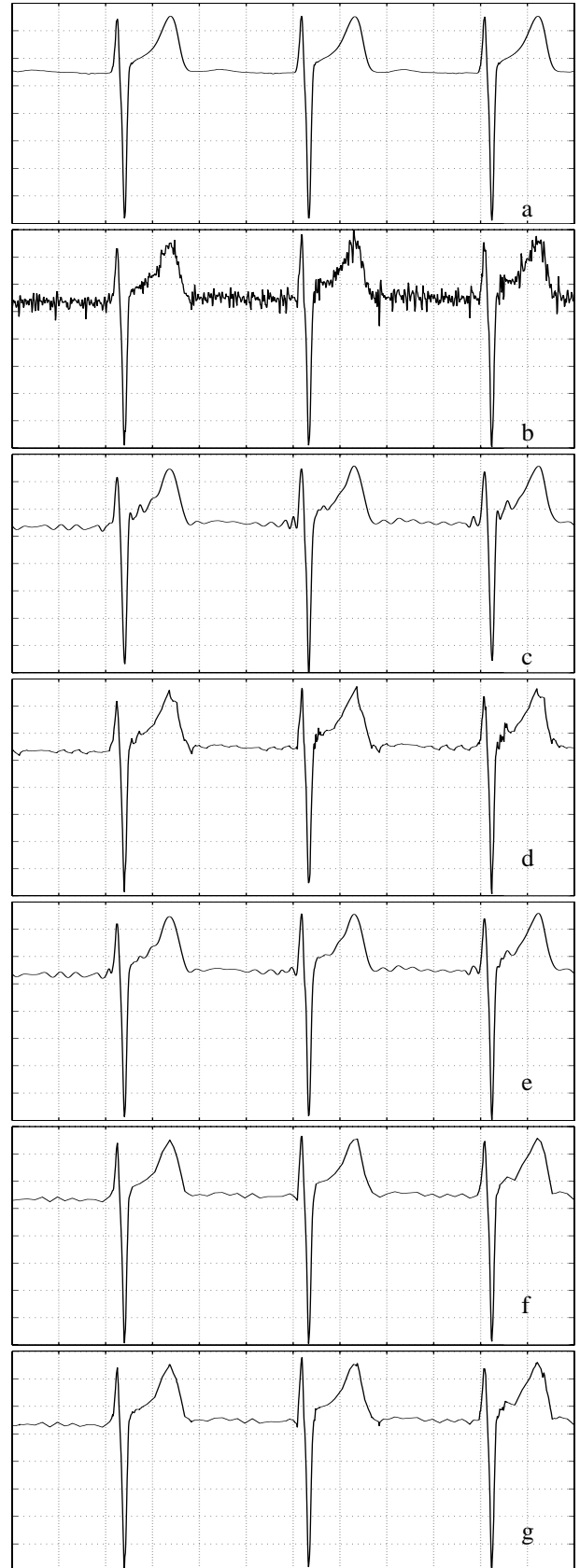
Figure 3. a) noise-free ECG; b) the same mixed with EMG; denoised with: c) C4 ( W_1 only); d) D2 ( W_1 only); e) Symlet10 ( W_2 only); f) Spline23 ( W_2 only); g) D2 ( W_1 ) and Spline23 ( W_2 ).
