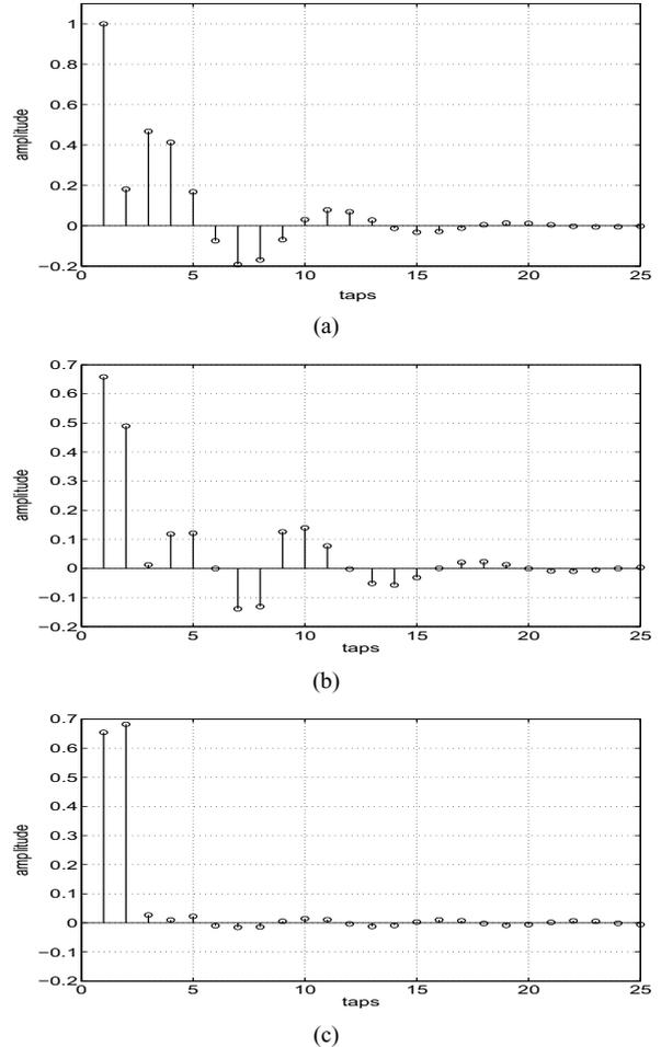
Figure 2: Impulse responses of (a) the original channel, (b) the equalized channel using an FIR filter of length eight, (c) the equalized channel using the proposed IIR filter with four zeros and three poles.
