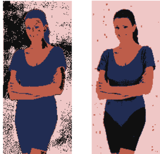
Figure 5. (a) Segmentation results in space using kmeans and 4 clusters, (b) same results using an additional local density feature defined using the MST.
