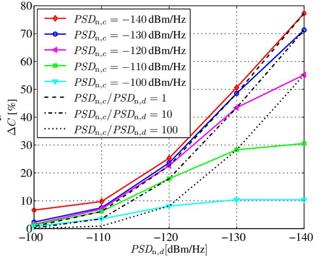
Figure 4: Capacity gain  $\Delta C$  as a function of the background noise PSD levels  $PSD_{n,d}$  at the DM port and  $PSD_{n,c}$  at the CM port in *downstream* direction for a 0.6mm loop of length  $L_{\text{loop}} = 1000\text{m}$  with a single equal-power FEXT disturber ( $N_{\text{FEXT}} = 1$ ) located at a distance  $L_{\text{xt}} = 100\text{m}$ . The non-solid lines show the capacity gains for constant ratios  $PSD_{n,c}/PSD_{n,d}$ .
