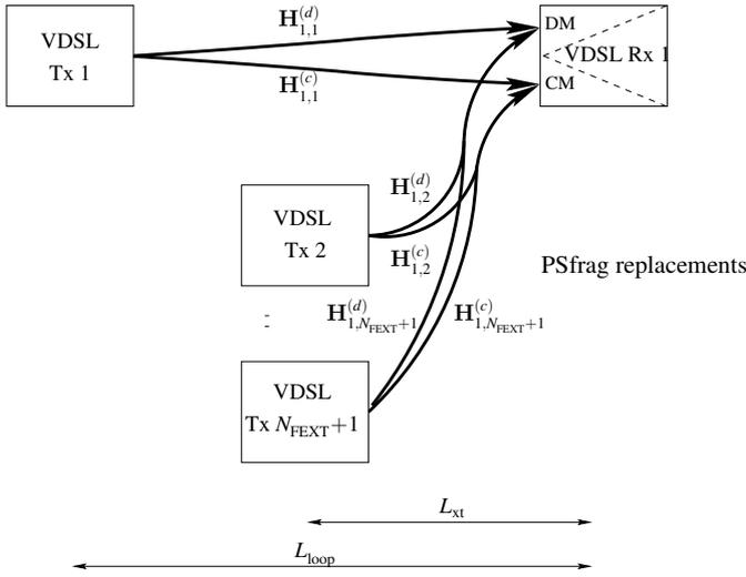
Figure 2: Simulation setup: VDSL transmission over a pair of length  $L_{\text{loop}}$  with  $N_{\text{FEXT}}$  self-FEXT disturbers located at a distance  $L_{\text{xt}} = 100\text{m}$  from the receiver. The convolution matrices correspond to the model (1) with  $k = 1$ .
