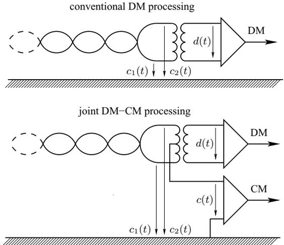
Figure 1: Conventional DM processing and joint DM-CM processing.
