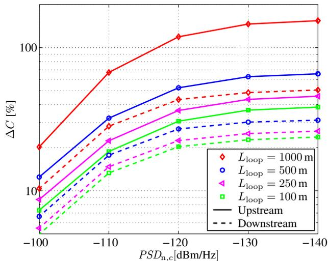
Figure 6: Capacity gain  $\Delta C$  versus CM background noise PSD level  $PSD_{n,c}$  for different loop lengths  $L_{loop}$  and a single FEXT disturber in upstream (solid lines) and downstream (dashed lines) direction ( $N_{FEXT} = 1$ ,  $PSD_{n,d} = -130$  dBm/Hz,  $L_{xt} = 100$  m).
