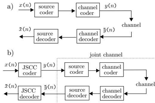
Figure 1: Separate and joint source-channel image transmission schemes
