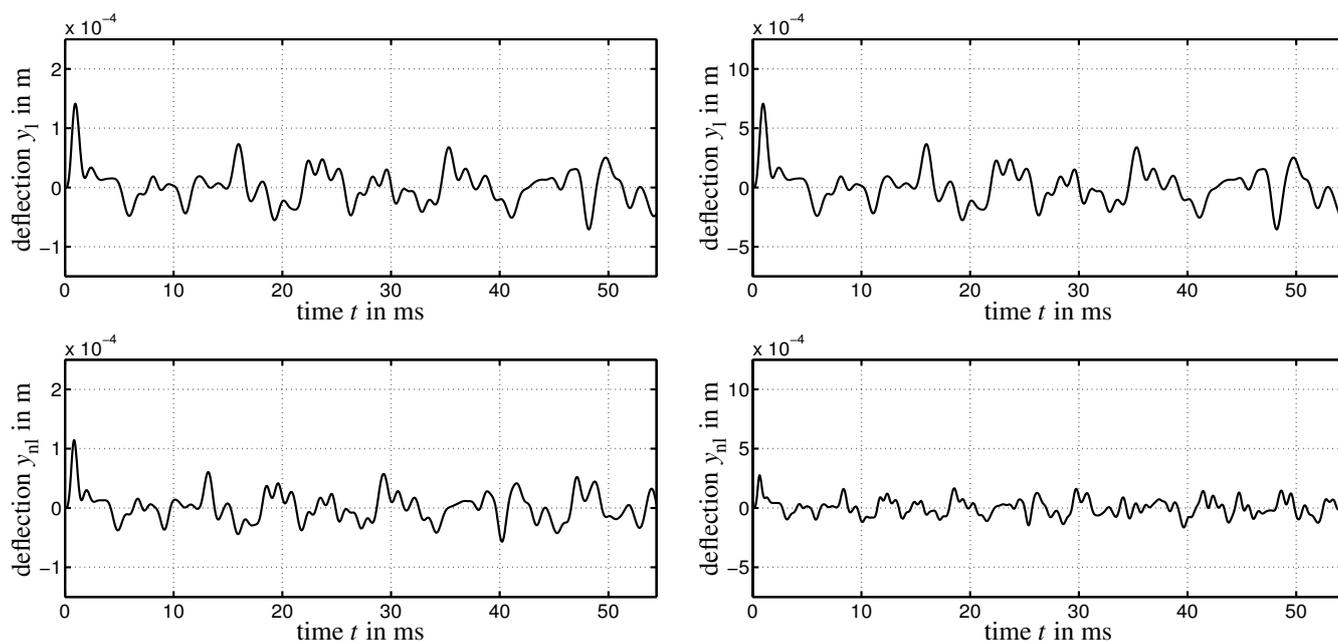
Figure 3: Simulation of a membrane’s deflection after it was excited by a band-limited impulse. The upper plots are the simulations of a linear model without tension modulation. The lower plots are the simulations of the same model with tension modulated nonlinearities. The simulations on the right were excited five times stronger.
