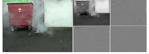
Figure 2: Frame with smoke and its single level wavelet subimages. Blurring in the edges is visible.
