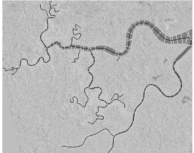
Figure 4: Unsupervised extraction of hydrographic network from a radar satellite image (ERS) using a hierarchical model. The black and white lines respectively correspond to the central axis and the successive widths of the extracted objects.
