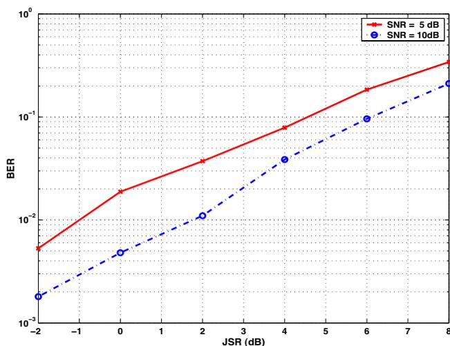
Figure 4: BER vs JSR for uplink transmission.
