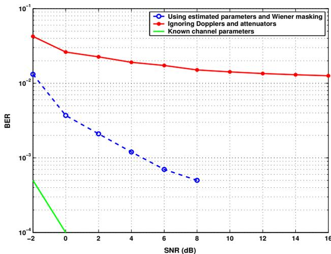
Figure 3: BER vs SNR for uplink transmission.
