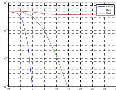
Figure 5: Comparison of BER on AWGN, CM1 and CM4 channel models (the synchronization is used and Detection Threshold = 0.1)
