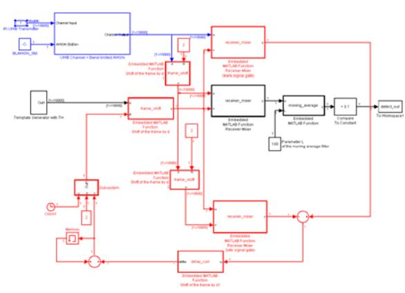
Figure 2: Simulink receiver model with early-late synchroniser.
