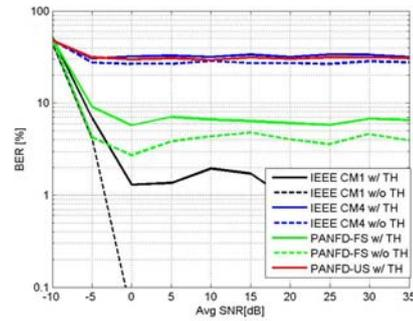
Figure 4– BER performance for single user system - multipath radio channels with and without time-hopping - a relative threshold of -16dB.
