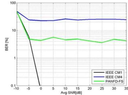
Figure 6 – BER performance for single user system- CM1, CM4 and PANFD radio channels with the receiver using the early-late synchronisation loop - without time-hopping - a relative detector threshold of -16dB.
