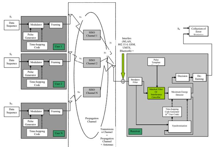
Figure 1: Schematic block diagram for the IR UWB multiuser system
