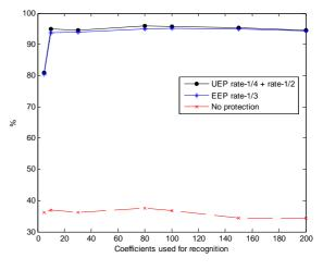
Fig. 5. Recognition rates for AWGN at  $E_b/N_0 = 3$  dB.
