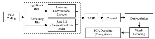
Fig. 1. Block Diagram of the System.
