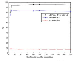
Fig. 7. Recognition rates for Rayleigh fading,  $E_b/N_0 = 3 \text{ dB}$ .
