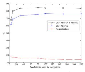
Fig. 4. Recognition rates for AWGN channel,  $E_b/N_0 = 0$  dB.
