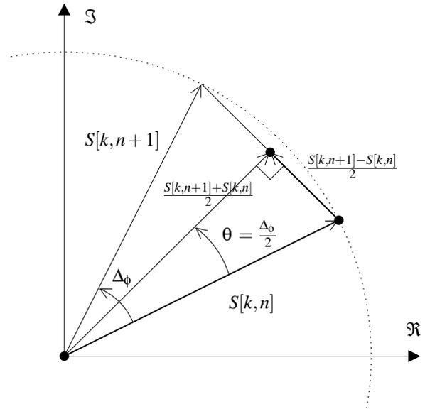
Figure 1: Vector relationships for phase difference and discrete derivative methods.  $S[k,n]$  is the spectrum at DFT bin number  $k$  and time index  $n$ , and  $\Delta_\phi$  is the phase difference between two consecutive (short-term) spectra.
