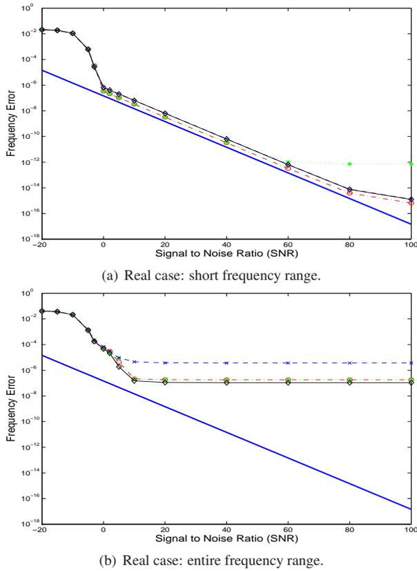
Figure 3: Performance of the tested estimators for the analysis of a real sinusoidal signal with frequency lying in the  $]0, 0.24[$  normalized frequency range (a), and in the  $]0, 0.5[$  range (b): the reassignment method (dotted line with \*), the difference estimator (dash-dotted line with  $\circ$ ), the derivative estimator (dashed line with  $\times$ ), and the trigonometric estimator (solid line with  $\diamond$ ). The CRB is plotted with a double solid line.
