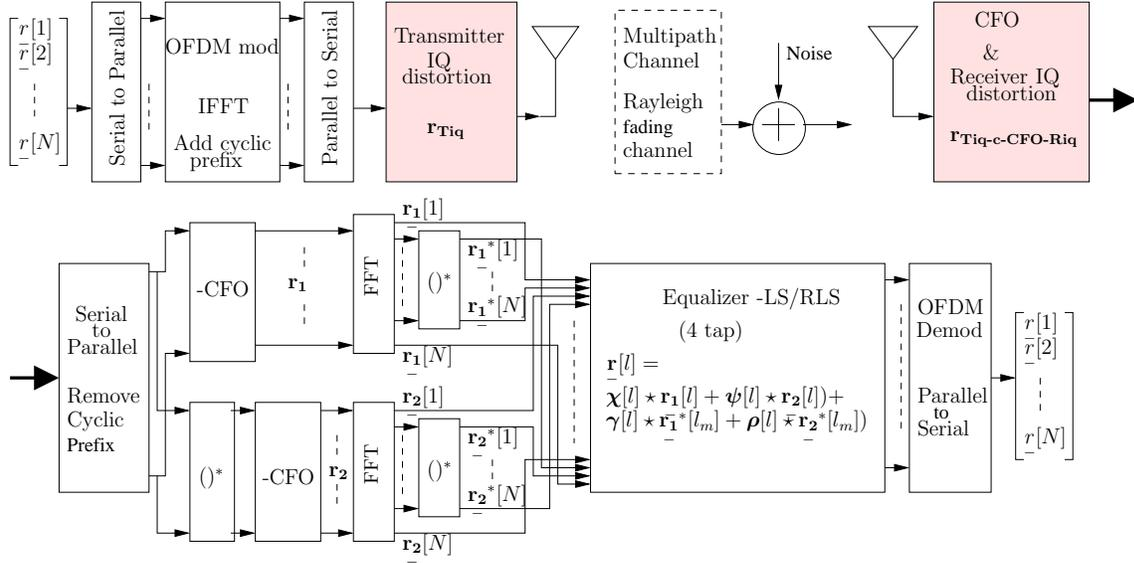
Figure 1: OFDM system with post-FFT compensation of transmitter and receiver IQ imbalance with CFO.
