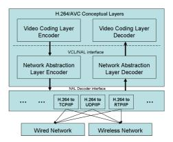
Figure 4: H.264/AVC standard in transport environment.
