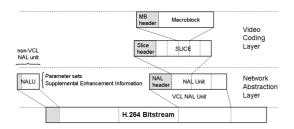
Figure 2: H.264 bistream encapsulation
