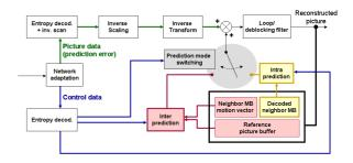
Figure 1: H.264 macroblock based decoding
