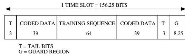
Figure 1: SCH slot structure.
