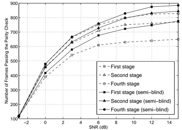
Figure 5: Number of frames passing the parity check (simulated GSM data).
