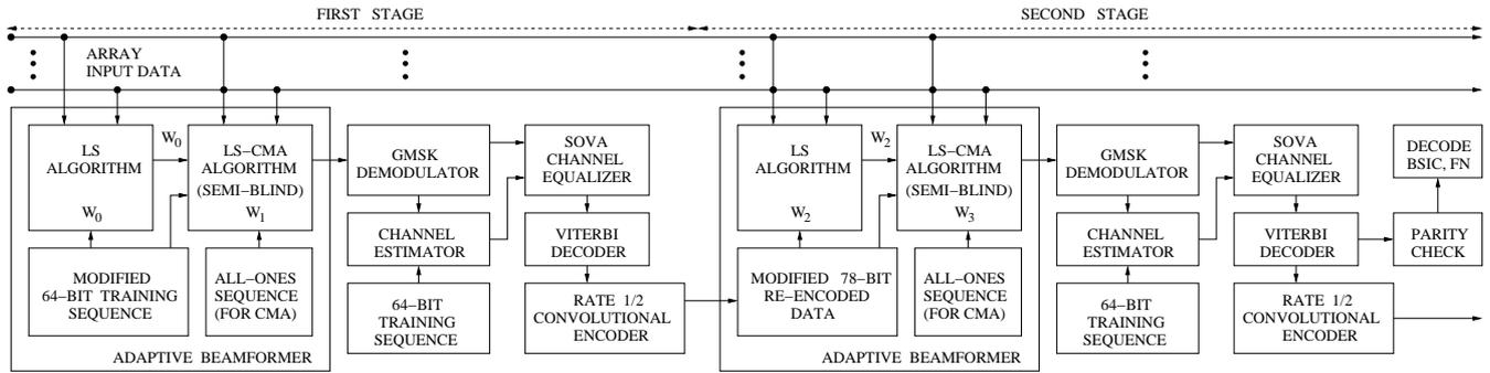
Figure 2: Iterative semi-blind receiver.
