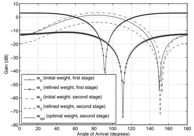
Figure 7: Beampatterns using the stochastic model.
