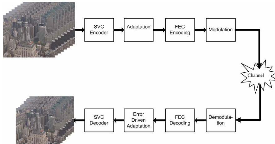
Figure 1. Communication chain for scalable video transmission
