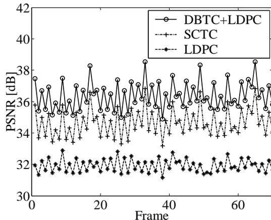
**Figure 5. . PSNR\_Y performance for different frame of City QCIF sequence at 300kbps at low  $E_b/N_o = 1.2$  dB.**
