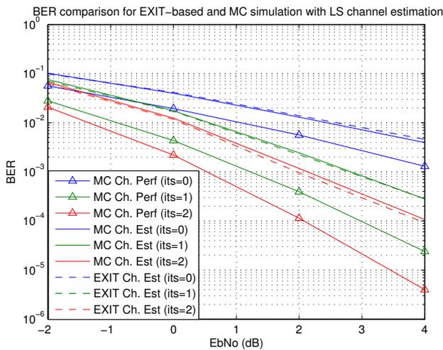
Figure 4: Comparison of EXIT function-based and MC simulation with LS channel estimation and a  $4 \times 16$  training matrix.
