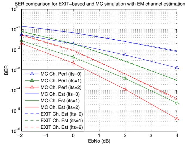
Figure 5: Comparison of EXIT function-based and MC simulation with soft decision-directed EM channel estimation and an initial  $4 \times 8$  training matrix.
