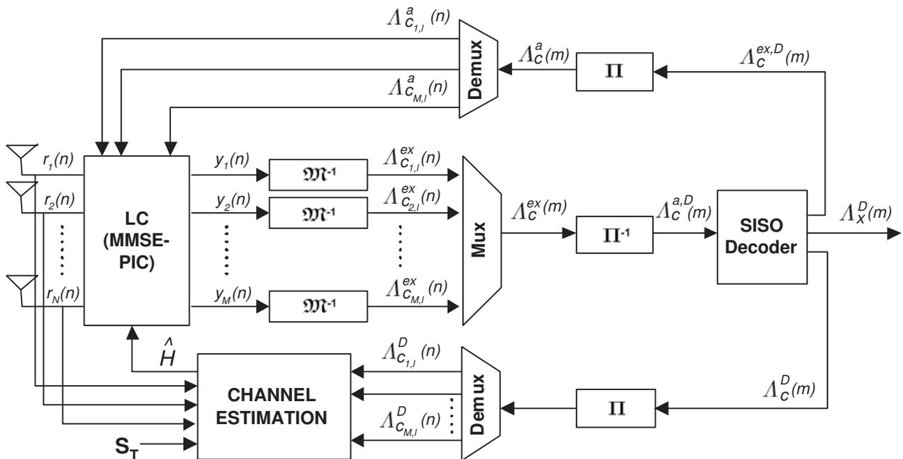
Figure 2: Diagram of a generic interference cancellation-based iterative MIMO receiver with channel estimation.
