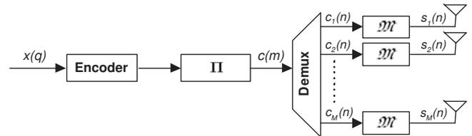
Figure 1: Diagram of a MIMO transmitter with coding and interleaving.
