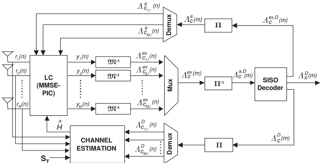
Figure 2: Diagram of a generic interference cancellation-based iterative MIMO receiver with channel estimation.
