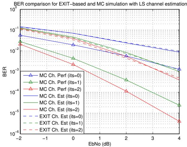
Figure 3: Comparison of EXIT function-based and MC simulation with LS channel estimation and a  $4 \times 8$  training matrix.
