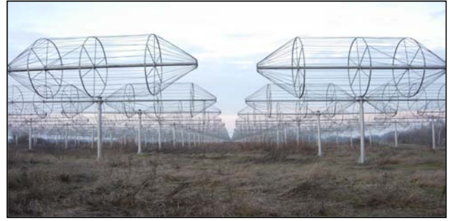
Figure 2 – Overview of the UTR-2 radio telescope, located near Kharkov (Ukraine). It is a T-shape phased array with 2040 dipoles. Its effective area is around \sim 140000 m 2 . Its frequency range of operation is 7 MHz to 32 MHz.
