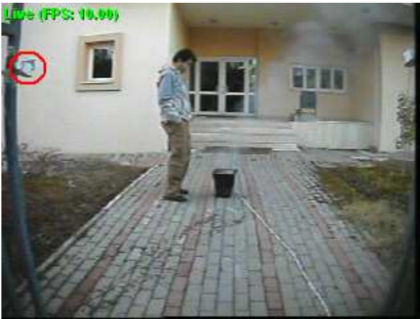
Figure 7: The PIR sensor is encircled. The fire is close to die out completely. A man is also within the viewing range of the sensor.
