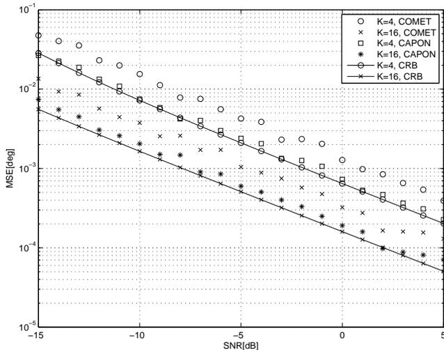
Figure 1: Angle MSE of the target located at  $\theta_1$ . The number of available snapshots is 100.
