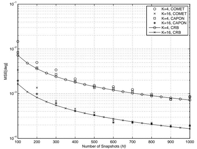
Figure 2: Angle MSE of the target located at  $\theta_1$ . SNR =  $-10$  dB.
