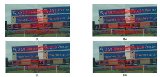
Figure 7: Keypoints matching using (a) SIFT (96 matches) (b) SIFT-RANSAC (83 matches) (c) SIFT-BP (48 matches) and (d) the proposed method (48 matches).
