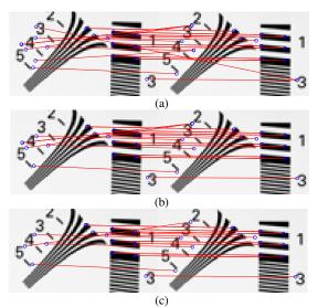
Figure 2: Keypoints matching of the original low resolution images (a) using original SIFT (25 matches) (b) using SIFT-RANSAC (23 matches) (c) using SIFT-BP (21 matches).
