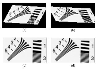
Figure 5: Results of super resolution for (a) SIFT (b) SIFT-RANSAC (c) SIFT-BP (d) the proposed method.
