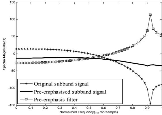
Figure 1 – Spectral magnitudes of a subband signal, pre-emphasis filter and pre-emphasised subband signal
