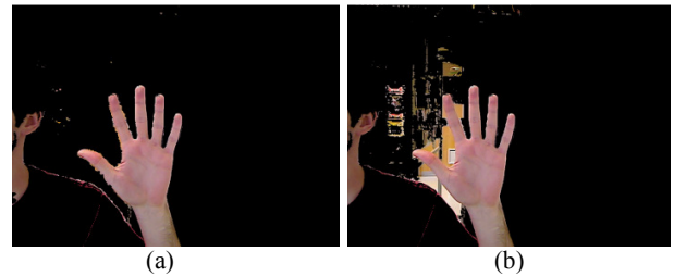
Figure 3 – Skin color detection results in the: (a) foreground image; (b) captured frame.
