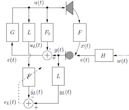
Fig. 2. AFC set-up with prefiltering of the loudspeaker and microphone signal
