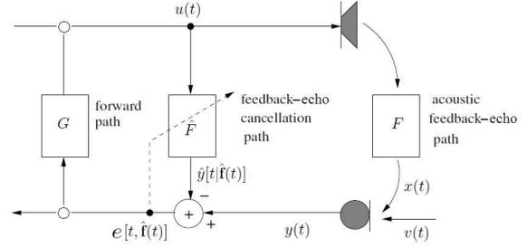
Fig. 1. AFC or AEC general set-up
