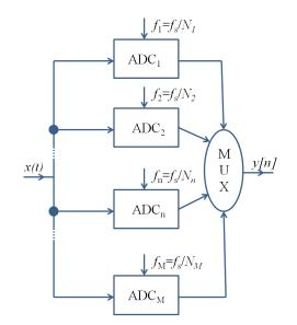
Fig. 2. Block diagram of a synchronous multirate system.
