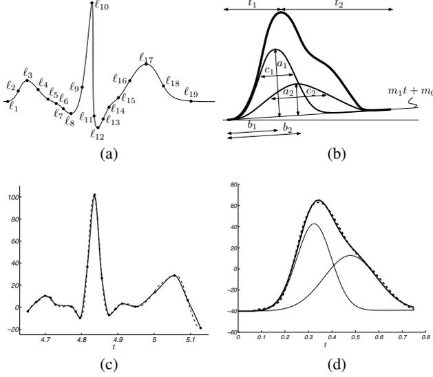
**Fig. 3.** Schemes for the parametrization of ECG (a) and PPG (b) pieces of one beat. Real examples of the shape model fitting for ECG (c) and PPG (d) pieces of one beat. Continuous line is the given by the model. Dashed line represents the original signal.
