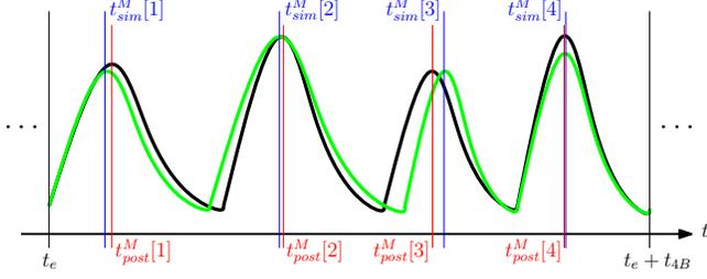
**Fig. 5.** Diagram of the methodology for the computation of the temporal error. The original piece  $—x_{post}(t)—$  is plotted in black, whereas the green line represents the synthetic piece  $—x_{sim}(t)—$ .
