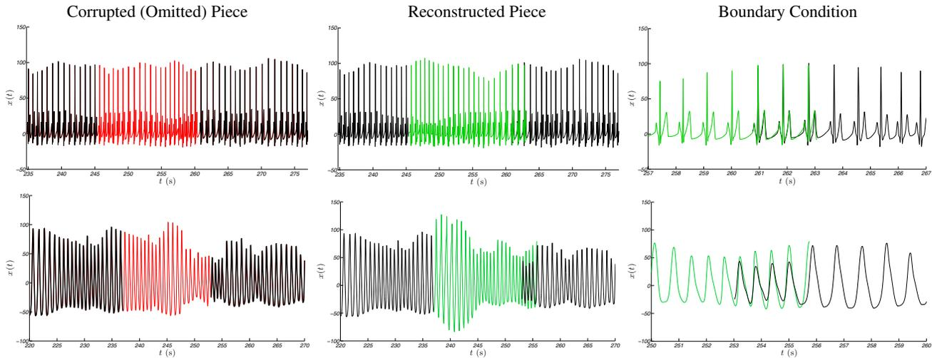
**Fig. 7.** Corrupted piece, reconstructed piece (with the optimal simulation), and zoom in on the boundary condition for ECG (top row) and PPG (bottom row).
