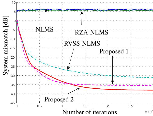
**Fig. 2.** Comparison of system mismatch (under impulsive noise).
