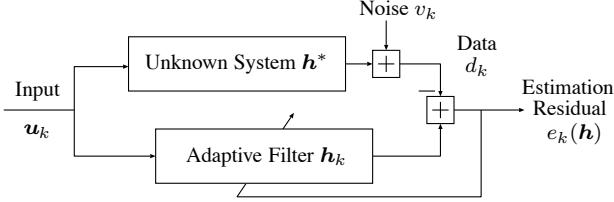
**Fig. 1.** Adaptive filtering scheme.
