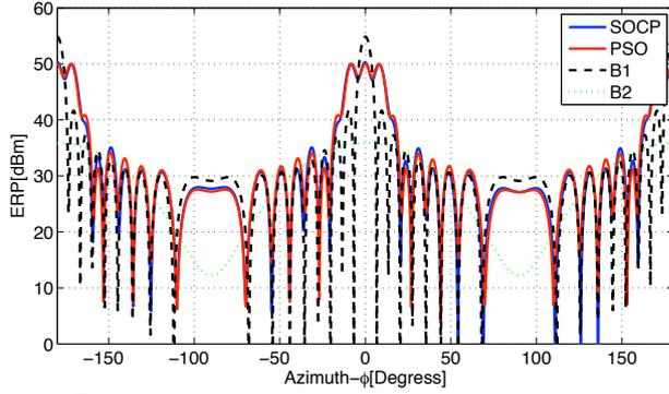
**Fig. 3.**  $\bar{\theta} = \pi/2$  cut of ERP computed for the beam patterns generated by SOCP (blue) and PSO based (red) methods for  $[\bar{\phi}_1, \bar{\phi}_2] = [-10, 10]$  degrees interval. High ERP narrow beam (B1-black) and low ERP wide beam (B2-green) are also provided.
