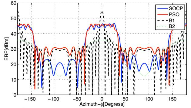
**Fig. 5.**  $\bar{\theta} = \pi/2$  cut of ERP computed for the beam patterns generated by SOCP (blue) and PSO based (red) methods for  $[\bar{\phi}_1, \bar{\phi}_2] = [-25, 25]$  degrees interval.
