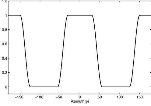
**Fig. 2.** Normalized magnitude of the spatial mask  $M(\phi)$  for azimuth interval  $[\bar{\phi}_1, \bar{\phi}_2] = [-30, 30]$  degrees.
