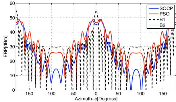
**Fig. 4.**  $\bar{\theta} = \pi/2$  cut of ERP computed for the beam patterns generated by SOCP (blue) and PSO based (red) methods for  $[\bar{\phi}_1, \bar{\phi}_2] = [-15, 15]$  degrees interval.
