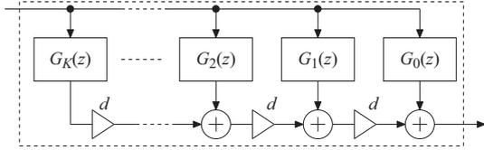
**Fig. 2.** Realization of  $G(z, d)$  used in Fig. 1.
