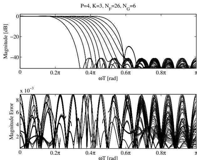
**Fig. 3.** Modulus of the frequency response (upper) and error  $E(j\omega T, b, d)$  (lower), for the Example 1 filter. Note that the modulus is the same for  $d$  and  $-d$  due to conjugate symmetry. Note also that the bumps seen in some of the magnitude responses occur in the transition region which is acceptable.
