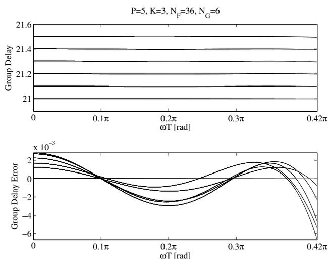
**Fig. 4.** Group delay (upper) and group delay error (lower), in the passbands, for the Example 2 filter.
