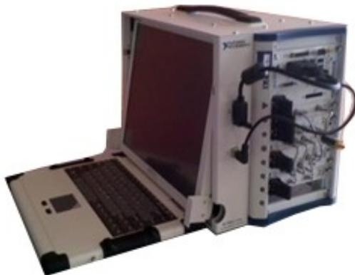
**Fig. 2.** Mobile eavesdropping system
