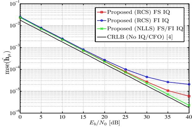
**Fig. 2:** MSE of channel estimation using (10), (16) and (11), in the presence of IQ imbalance and normalized CFO with  $N=64$ , Rayleigh channel with  $L_h=6$  taps.
