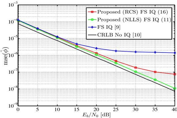
**Fig. 3:** MSE performance of CFO estimation with (11) and (16) with  $N=64$ , Rayleigh channel with  $L_h=6$  taps.
