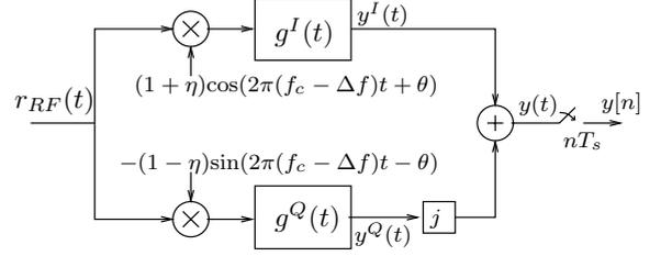
**Fig. 1:** The equivalent model of a DCR in the presence of FS IQ mismatch and CFO.
