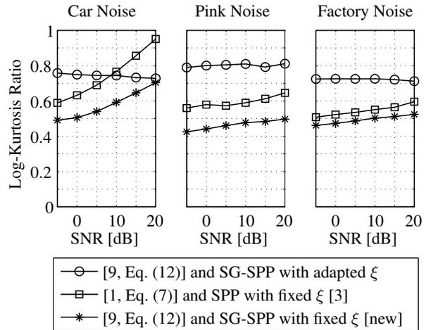
**Fig. 3.** Evaluation results of speech enhancement approaches based on an MMSE-STSA weighting rule and an SPP estimator w. r. t. amount of musical noise based on the log-kurtosis ratio (the lower the value the less the amount of musical noise) [16]
