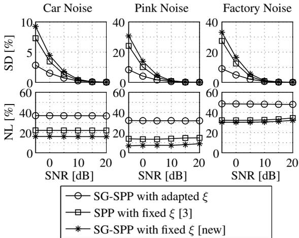
**Fig. 2.** Evaluation results of the reference and the proposed SPP estimators w. r. t. NL and SD [3]
