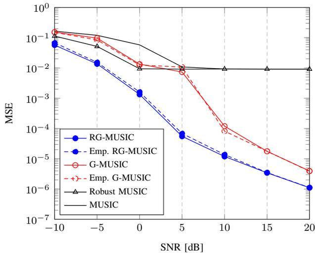
**Fig. 1.** Mean square error (MSE) performance of the smallest angle estimation of the MUSIC estimators for  $N = 20$ ,  $n = 100$ , two sources at  $10^\circ$  and  $12^\circ$ , Gamma-(0.8, 1.25) impulsions. Robust G-MUSIC (RG-MUSIC) and empirical robust G-MUSIC (Emp. RG-MUSIC) are compared against MUSIC, G-MUSIC, and empirical G-MUSIC (Emp. G-MUSIC).
